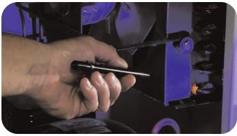
For the HVAC contractor, the titanium TT-3C UV model will fluoresce the majority of dyes used for leak detection. The black TT-3C UV model illuminates a broader range of dyes and is used primarily in law enforcement.
